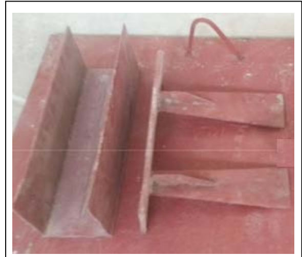
Figure 5 Strip footing model and loading blades
