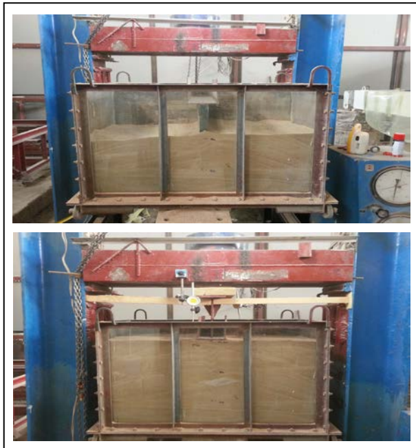
Figure 7 Plane strain piles model test under strip footing, (Piled-strip)
