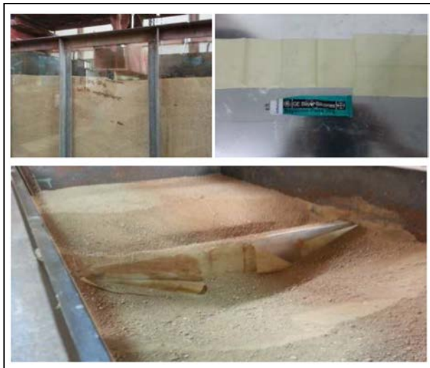
Figure 11 Details of end bearing piled-strip model test
